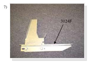
Attach one 3124F to each bracket using 5/16 bolts and nuts. Snug but do not tighten.
