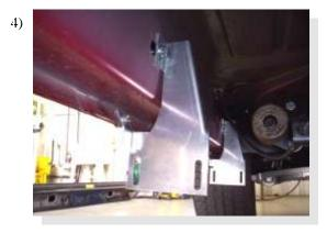
Attach brackets to vehicle by inserting the retaining nut in the factory obround hole and using one 5/16" bolt and nut through the pinch weld. Use the FL148 brackets in the forward locations and the FL149 In the rear most location. (No FL149 is used or included for Std cab models).
