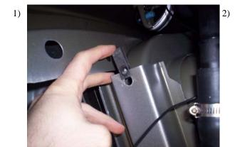
Locate the front bed cross member and install clip nut as shown in **Fig. 1.**
