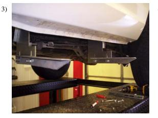
Attach a 3124F angle bracket to the FL181 bracket with 5/16" bolts and nuts. Snug but do not tighten at this time. **Picture shows long bed with extra bracket not needed in short bed.**
