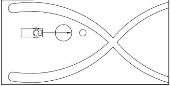
**3.** Remove plastic plug from under body at 77" location and install clip nut as shown.
