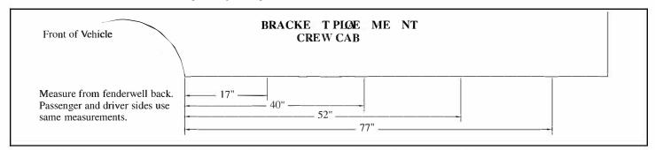
2. Measure from front wheel well, back to dimensions shown above. Mark these bracket location centers.
