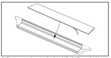
**6.** Place step pad on running board. Peel off tape backing to secure. Install the Owens logo.
