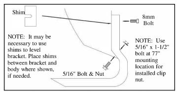
**4.** Attach brackets to measured locations using 5/16" bolt and nut at factory pinchweld holes, and 8mm bolt into factory nut.
