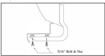
**5.** Position board on brackets. Use proper slot to center board under doors. Attach with 5/16" bolts and nuts.
