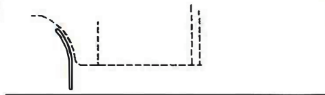
④ BEND STONE GUARD BY HAND AND KNEE TO FIT THE WHEEL WELL BEFORE INSTALLING TO RUNNING BOARD
