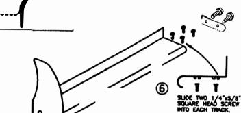
FASTEN FRONT STONE GUARD TO BOARDS WITH 3/8" SELF TAPPING BOLT. BEND STONE GLAND BY HAND AND KNEE TO FIT THE WHEEL WELL
