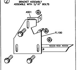
BRACKET ASSEMBLY MOUNT TO BODY PREDRILL A 5/16" HOLE THROUGH THE PINCH WELD. ATTACH FL100 BRACKET TO THE BODY WITH 5/16" BOLT AND NUT, LOOSLY TIGHTEN. ATTACH THE ASO1 BENT TAB TO THE BODY PANEL WITH A \$14x 3/4" SELF DRILLING SCREW.
