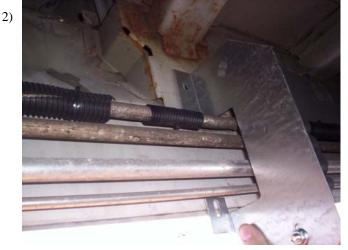
Attach the FL199 for 2" riser boards or the FL201 for the 4" riser boards by inserting either an 8mm bolt through the top hole in the bracket into the pull nut, or, if there is no hole for the pull nut, use the self drilling screw. Insert 5/16" flanged bolt through the hole in pinch weld and through slot in FL199 and tighten. Follow the rest of the steps in the other instruction sheet for board installation.
