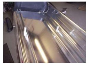
Insert one square head bolt into front & rear track for each bracket.
