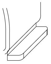
HOLD THE BOARD IN PLACE WITH IT RESTING ON THE BRACKETS.
