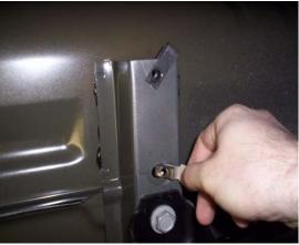
In front of rear wheel, above front leaf spring shackle, on the bed cross member, attach clip nut and 8mm pull nut, as shown in **Fig. 4.**
