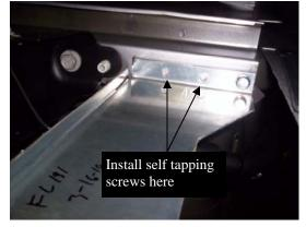
Attach the FL221 bracket to the front bed cross member support, using 5/16" bolt, as shown in **Fig. 2.** Next install self tapping screws into the other holes in the bracket to the cross member.
