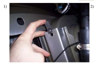
Locate the front bed cross member and install clip nut as shown in **Fig. 1.** If no hole is present you will have to drill a 1/2" hole and insert 8mm pull nut as shown in **Fig. 4**
