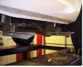
Attach a 3124F angle bracket to the FL181 and FL180D & P with 5/16" bolts and nuts. Snug but do not tighten at this time.
