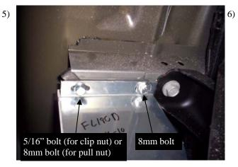
Install FL180D & P using 5/16" flanged bolt (for clip nut only) and 8mm bolt and washers, as in **Fig. 5.**
