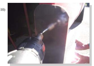
Make sure board is lined up with cab board. Use one self drilling screw to attach the stone guard to the fender lip. Make sure the board is level, then use remaining 2 screws to finish attaching stone guard to fender lip.
