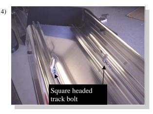
Insert one square headed track bolt into tracks for each bracket.
