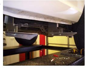
Attach a 3124F angle bracket to the FL221 bracket with 5/16" bolts and nuts. Snug but do not tighten at this time. **Picture shows long bed with extra bracket not needed in short bed.**
