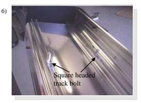
Insert one square headed track bolt into each for each bracket.
