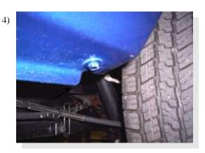
Remove the factory fender brace bolt but do not discard. This will be re-installed to hold the board.
