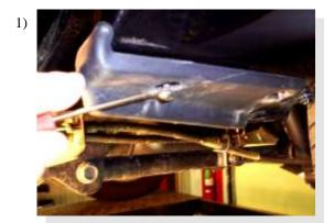
Remove the plastic edge protector on the front edge of the box. To remove, use a small screw driver to pull out the push pin. Remove and discard.
