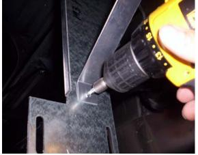
Attach FL198D/P to FL193D/P with a self tapping screw as shown In **Fig. 6.** Make sure brackets are strait and tighten fender support nut.
