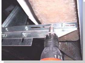
Using self drilling screws attach the board to the angle brackets. Using 1-1/4 self tapping screw attach board to bed close to the wheel well.
