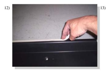
Apply foam tape to the top lip of the board. Apply the step tread also at this time.
