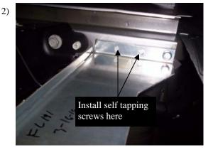
Attach the FL192D/P bracket to the front bed cross member support, using 5/16" bolt, as shown in **Fig. 2.** Next install self tapping screws into the other holes in the bracket to the cross member.
