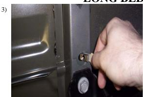
Hold FL193D/P up to rear bed cross member and make a mark in the front and rear hole of the bracket on the cross member. Drill a 1/2" hole at each mark and insert a pull nut into each hole, as shown in **Fig 3**. Install self tapping screws into remaining holes.
