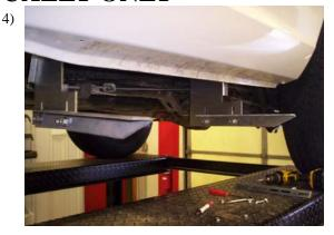
Attach a 3124F angle bracket to the FL192D/P and FL193D/P, with 5/16" bolts and nuts. Snug but do not tighten at this time. "Dually only" attach 3124G to FL193D/P.
