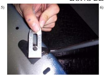
Remove fender support nut located on front of rear wheel well. Attach FL 198D/P and snug nut.
