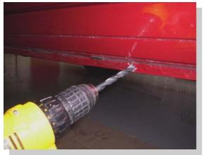
Drill a 5/16" hole in pinch weld at pre-marked location, to insert a 5/16" flanged bolt through pinch weld and FL223 and FL232.
