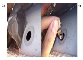
Remove tape from underbody to install 8mm pull nut at 22" 38" DR side, and 7" 19" 36" 49" pass side.
