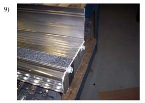
Attach the end caps to the board with 3/8" self threading bolts. (extruded board shown)
