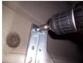
At remaining locations install two self tapping bolts through slot in FL223 (**Different BRKT shown**)
