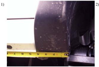
Measure from front wheel well back making a mark on the pinch weld at (Pass side 10", 22", 38", 50", 70", 88" 100") (DR side 7", 19", 36", 49")
