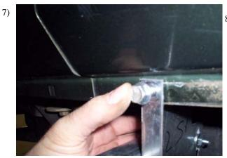
Insert a 5/16" flange bolt trough pinch weld and FL223 and FL232 tighten with a 5/16" flanged nut. (BRKT show on outside of pinch weld for picture purpose only, BRKT mounts to inside of pinch weld)
