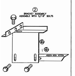
BRACKET ASSEMBLY MOUNT TO BODY ASSEMBLE WITH 5/16" BOLTS AND \$14 SELF DRILLING SCREWS
