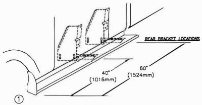
MEASURE FROM FRONT WHEEL WELL TO BRACKET LOATIONS, MARK THIS DIMENSION ON THE PINCH WELD
