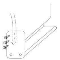
Level board and attach stone guard to vehicle using the sheet metal screws that are included or drill holes in the stone guard in the locations of the screws removed from the OEM plastic stone guard.
