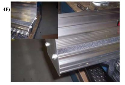
Attach the stone guard and end caps to the board with 3/8" self threading bolts. (extruded board shown)
