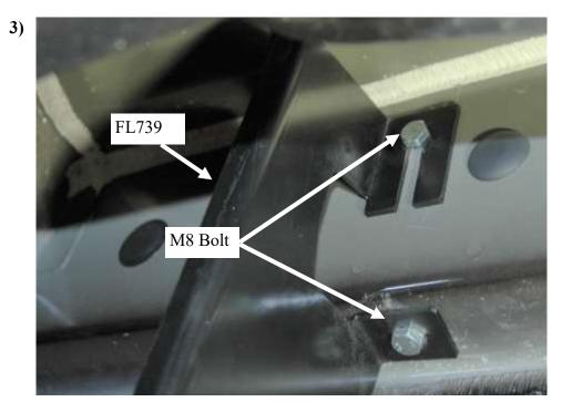
Attach brackets to vehicle by inserting a M8 x 20 mm bolt into each of the threaded holes in back of rocker. Tighten bottom bolt first then the top bolt. For each bracket location.
