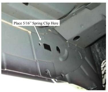
At each of the measurements above slide 5/16" spring clips supplied in bolt package into the larger hole slide toward the smaller hole until clip snaps into position.
