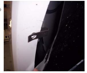
Pull inner plastic wheel well cover back and install clip nut into hole where push pin was.
