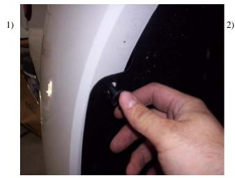
Start by removing push pin in rear inner plastic wheel well cover.
