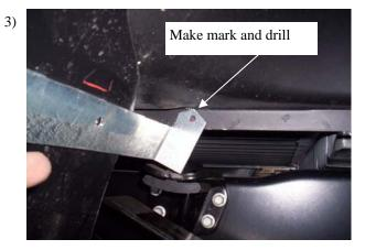
Insert a 5/16" flanged bolt through first hole in the bracket to help hold in place. Then place bracket against pinch weld on bed and make a mark; drill a 5/16" hole.
