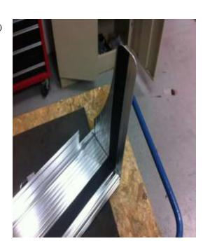
Prepare the running board for installation. Slide square head bolts into each track located on the bottom side of the board. **Fig 7**These will be used to attach the board to the previously mounted brackets. Next attach mud flaps to front end and end cap to rear of board. **Fig 8** Tread tape should face in-word and match with tread tape on the running board.
