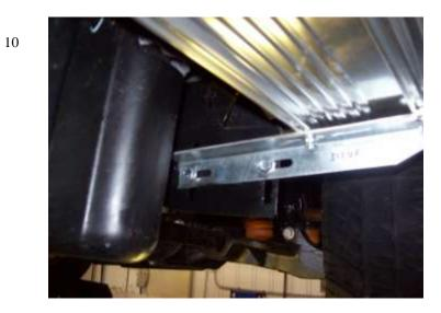
Secure the running board to the brackets with 1/4" nuts. Making sure one last time the running board is level tighten the nuts on the bolts to secure the board. **Fig 10**
