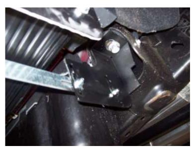
On passenger side in front and behind the Diesel DEF tank remove the cab mounting bolt with 18mm socket, slide bolt through top hole of FL508 bracket **Fig 6**, making sure the FL508 is straight when tightening. Then bolt the 3124F onto FL508 with two 5/16 bolts and nuts.
