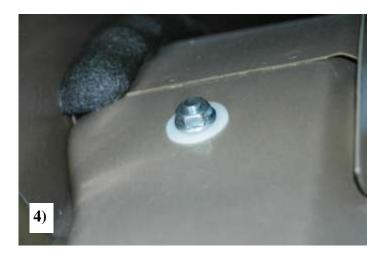
With the 5/16" x 3/4" flange bolt through the bracket and plastic washer, slide through the rear wheel well slot. On the back side of slot place a <u>plastic</u> <u>washer</u> onto the threads protruding through the wheel well and put a 5/16" flange nut onto the threads.
