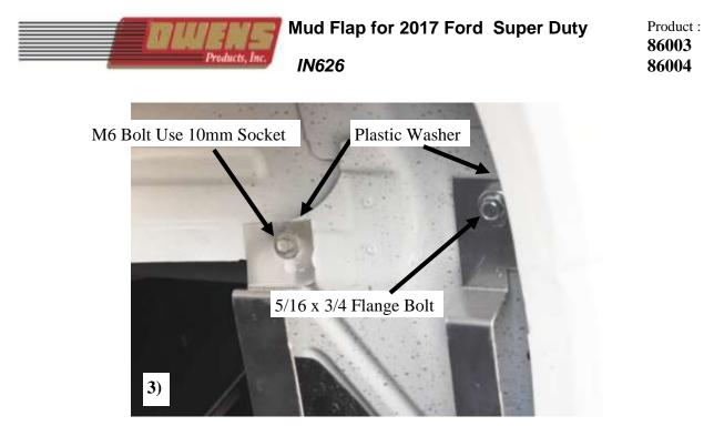
Remove the M6 bolt from just inside the rear wheel well. Place a <u>plastic washer</u> between the steel bracket and the aluminum body and install the M6 bolt that was removed into the slot on bracket, the slot is there to adjustment to level mud flap. Once the M6 bolt is snuged up to hold bracket, slide a 5/16" x 3/4" flange bolt through the other slot in bracket making sure that a <u>plastic washer</u> is in between the steel bracket and the aluminum body.
