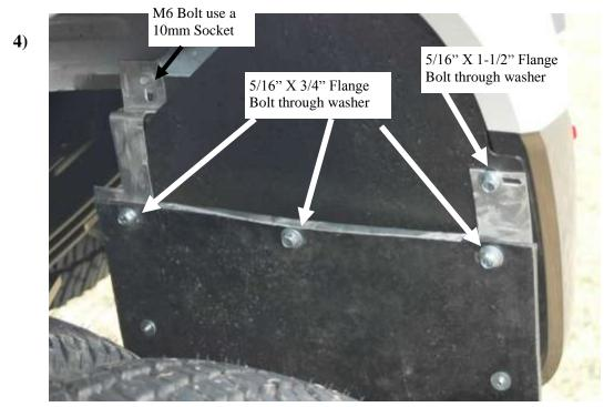
First drill through the rubber in each of the top slots of the mud flap with 5/16" drill bit. Then attach the bracket to the rubber mud flap with three 5/16" x 3/4" flange bolts through washers and install flange nuts to rear side of the bracket.
