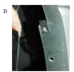
Pull inner plastic wheel well cover back and install clip nut into top hole where push pin was.
