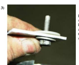
Remove the M6 bolt from just inside the splash shield that the push pin was removed in step 1. Place a plastic washer between the steel bracket and the aluminum body and install the M6 bolt that was removed into the slot on bracket, the slot is there to adjustment to level mud flap.
