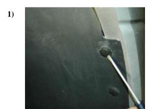
Start by removing push pins in rear inner plastic wheel well cover with a small flat blade screwdriver, pry out the center of the plastic rivet out to remove.
