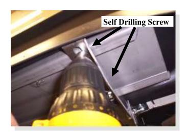
Place the board on the brackets and center up on the cab of the vehicle from front to rear. Attach to the brackets using #14 X 3/4" long self drilling screws into the shoulder of the steel channel on the bottom of the board.
