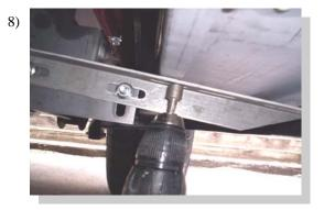
For plastic boards, place board on brackets to desired location. Attach by using 3/4" long self drilling screw into the steel support under the board.
