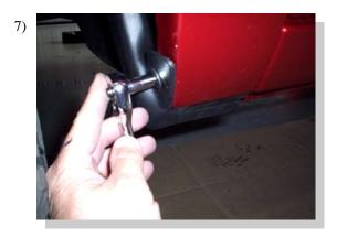
It may be necessary to remove the small stone guard in the front fender well. Test fit your board to see if it will need to be removed. If it does, remove the small screw holding it in place and then unsnap. Reinstall the screw.
