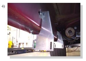
Attach brackets to vehicle by inserting the retaining nut in the factory obround hole and using one 5/16" bolt and nut through the pinch weld. Use the FL142 brackets in the forward locations and the FL143 In the rear most location. (No FL143 is used or included for Std cab models).
