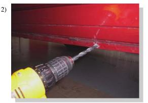
At each of the locations from step one, drill a 23/64" hole through the pinch weld.
