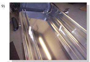
For aluminum boards, insert one square head bolt into track for each bracket.
