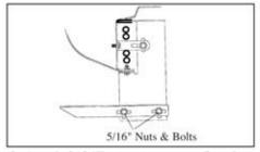
Attach 3124F step support to flat plate using two 5/16" nuts and bolts. Do not tighten at this time.
