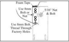
3. Place foam tape at top of FL130 flat plate. Bolt to AS02 then to pinch weld with 8mm bolts. Note: top of flat plate must hit rocker panel. Tighten to AS02 and 8mm bolt before tightening to pinch weld.
