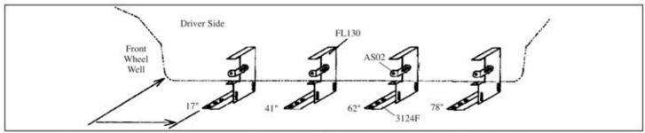
Measure from front wheel well, back 17", 41", 62", and 78". Mark these bracket locations. Note: Factory holes should be close
