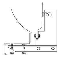
SECURE BOARD TO BRACKET WITH 1/4" NUTS
