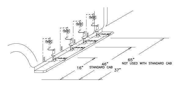
MEASURE FROM FRONT WHEEL WELL TO BRACKET LOCATION MARK THIS DIMENSION ON THE PINCH WELD
