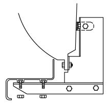
SECURE BOARD TO BRACKET WITH 1/4" NUTS
