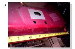
Measure from front wheel well back and make a mark at: 25",47",67",78" along the pinch weld.
