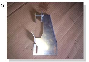
Assemble brackets as shown using one 5/16" bolt and steel retaining nut.
