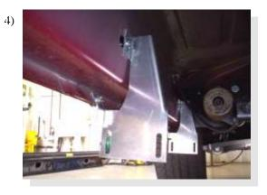
Attach brackets to vehicle by inserting the retaining nut in the factory obround hole and using one 5/16" bolt and nut through the pinch weld. Use the FL148 brackets in the forward locations and the FL149 In the rear most location. (No FL149 is used or included for Std cab models).
