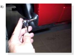
Remove the small factory stone guard in the front fender well by removing the small screw and then unsnap. <u>Reinstall</u> the screw.
