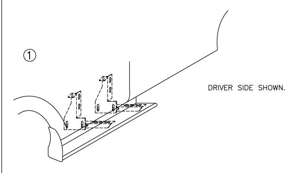
MEASURE FROM FRONT WHEEL WELL TO BRACKET LOATIONS. MARK THIS DIMENSION ON THE PINCH WELD
