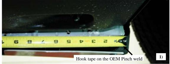
Measure back from front wheel well as seen in Fig 1, under side at the distance listed below.
