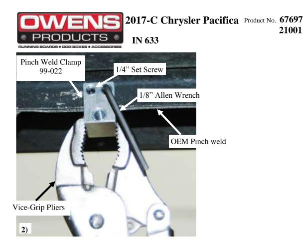
At each center mark, mount the pinch weld clamp 99-022. Tighten the set screws with 1/8" Allen wrench holding with pair of vise grips for leverage.
