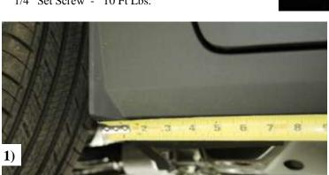
Measuring from the back side of the front mud flap as shown in photo. Mark the inside of pinch weld with marker. Driver side Positions: 1st = 12", 2nd = 39-1/2", 3rd = 62"
