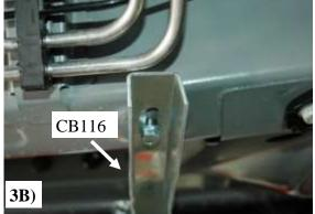
3) Mount a CB116 using a 5/16"x1-1/2" bolt through CB116 thread into <u>short</u> re-enforcement nut then slide nut into the hole in the frame. **Hole at 11 1/2" from front wheel well. (Photo 3A)**
