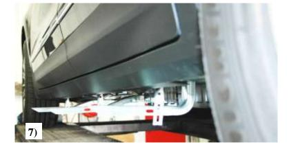
Place the board on the brackets and align from front to back and level the board. Tighten <u>all</u> loose bracket bolts now.
