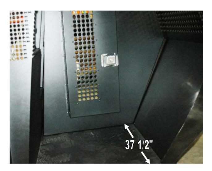
Once the K9 insert is mounted in vehicle. Slide the divider into the K9 insert so the door is on the driver side.
