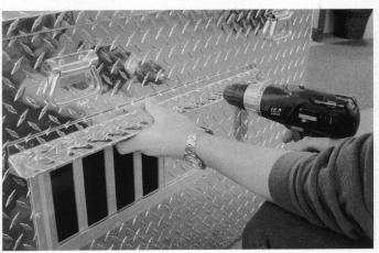
3. Using the pre-punched holes in the rain gutter as a guide, drill a 3/16" hole through the aluminum wall of the dog box. See illustration above.
