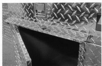
6. Center the 19" rain gutter above the dog compartment door. Make sure the rain gutter does not obstruct the door from opening before drilling. See illustration above. Follow steps 3-5 to complete the installation. Use the same procedure for the other dog compartment door.
