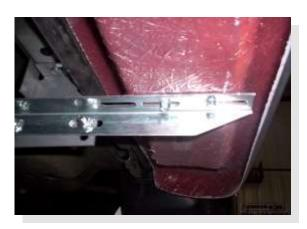
Place the board on the brackets and align up on the vehicle. There is a driver and a passenger side board. Attach to the brackets using #14 X 3/4" long self drilling screws, making sure you are drilling through steel mounting pad on under side of board.
