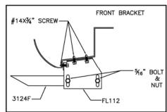
**4.** Attach FL112 to marked locations using #14 x 3/4" self-drilling screws into the pinch weld and the rocker panel.
