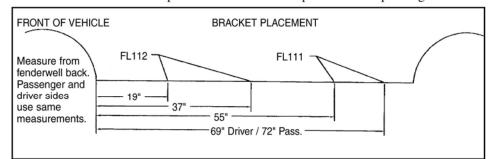
3. Measure from front wheel well, back to dimensions shown above. Mark these bracket location centers. Note: Steel plates have been inserted under fiberglass to mount brackets. Double check your marks to be sure they line up with the steel plates before drilling.
