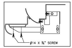
7. Position step on brackets. When proper placement is achieved, use #14 x 3/4" self-drilling screws to attach to brackets. Use 2 screws per bracket.
