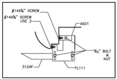
5. Bolt AS01 to FL111, just lightly tighten. Place flat bracket FL111 at the pinch weld locations shown above. Use 2 #14 x 3/4" self-drilling screws to attach the flat bracket to the pinch weld. Use another self drilling screw to attach the AS01 bent tab to the rocker panel. Tighten the 5/16" nut and bolt holding the bent tab to the flat bracket.
