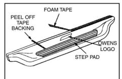
6. Clean surface prior to attaching tape and step pads with denatured alcohol. Apply foam tape to top lip of board. Position step pad on stepping surface. Peel off tape backing starting with rear strip. Keep pad in position, peel off backing then apply pressure to top of pad to stick tape to board. Continue above steps for all tape strips.
