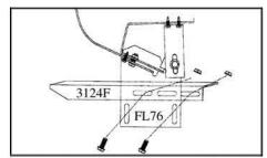
Attach 3124F step supports to FL76 using two each 5/16" nuts and bolts. Snug with fingers but do not tighten at this time.
