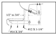
8. Position step on brackets. Align back of step upper lip approximately 1-1/2" out from edge of pinch weld. Use #12 x 3/4" screw through lip. (Note: If installing box boards, align both before securing steps to body.) Next, attach step to 3124F using two #14 x 3/4" screws. Adjust brackets and tighten all bolts to 18 foot pounds.
