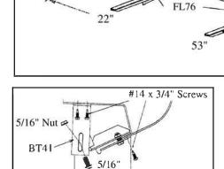
5A. Attach BT41s to FL76s using 5/16" nuts and bolts. Mate top of BT41s to bottom of step areas. Screw BT41 to bottom of step area using two #14 screws, then screw through FL76 into pinch weld using one #14 screw. Snug 5/16" nut and bolt.
