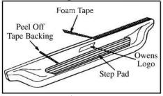
7. Clean surface prior to attaching tape and step pads with denatured alcohol. Apply foam tape to top lip of board. Position step pad on stepping surface. Peel off tape backing starting with rear strip. Keep pad in position, peel off backing then apply pressure to top of pad to stick tape to board. Continue above steps for all tape strips.
