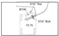
Mate BT40 top clamp onto FL76 flat plate using 5/16" nuts and bolts. Clamp assembly onto pinch weld at marks.
