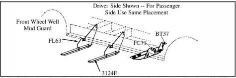
3. Steel plates have been inserted under fiberglass to mount brackets securely using self-drilling screws. See illustration at right. Follow instruction steps #5 and #6 for bracket locations.
