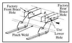
5. Mount FL63s to front and rear frame braces using 5/16" nuts and bolts through factory brace holes. Mount to back of forward most brace, and to front of rear most brace. Do not tighten bolts at this time.
