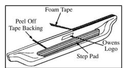
8. Clean surface prior to attaching tape and step pads with denatured alcohol. Apply foam tape to top lip of board. Position step pad on stepping surface. Peel off tape backing starting with rear strip. Keep pad in position, peel off backing then apply pressure to top of pad to stick tape to board. Continue above steps for all tape strips.
