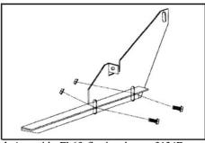
Assemble FL63 flat bracket to 3124F step support using two 5/16" nuts and bolts. Do not tighten at this time.
