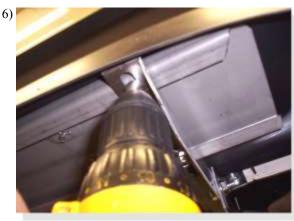
Position <u>running board</u> between wheel wells for best fit. Install self taping bolts through bracket into the shoulder of the steel channel on the bottom of the board.
