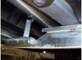
Insert M10 pull nut into frame rail, @ 20" then insert M10 bolt through FL259 thread into pull nut. Pull out rubber plug in rocker panel and insert 5/16" bolt through BT78 thread into re-enforcement nut, slide nut into hole on rocker and tighten up to rocker. Secure BT78 to FL259 with 5/16" bolt and nut.
