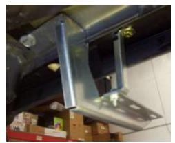
Insert 1/4" carriage bolt through pinch weld @ 64" remove bolt holding fuel tank strap. (Note: fuel tank will not move) Slide FL260 onto carriage bolt and replace fuel tank bolt through FL260 and tighten. Pull rubber plug from rocker and using BT78 repeat process like other 2 brackets.
