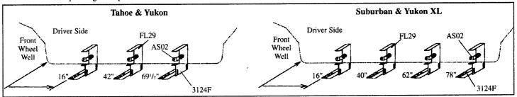
3. Measure from front wheel well, back to dimensions shown above. Mark these bracket locations.
