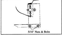
6. Attach 3124F step support to flat plate using two 5/16" nuts and bolts. Do not tighten at this time.
