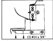
9. Secure step support bracket to bottom of step using two #14 x 3/4" self-drilling screws per bracket into the metal support. Tighten all bolts to 18 foot pounds.
