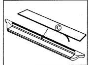
10. Tighten step support bolt and nut to 18 foot pounds. Place pad on step. Peel off tape backing to secure. Don't forget the Owens label!
