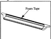
7. Apply foam tape to top edge of step. Remove protective strip from top edge of foam tape.
