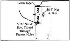
5. Place foam tape at top of FL29 flat plate. Bolt to AS02 then to pinch weld with 5/16" nuts and bolts. Note: top of flat plate must hit rocker panel. Tighten FL29 to AS02 and 8mm bolt
