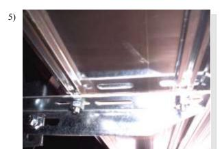
Insert one square head bolt into each track for each bracket. Set board on brackets with 1/4" bolts going through slots on bracket, attach with the 1/4" nuts. Level board and tighten down any and all loose nuts and bolts. Repeat for the other side.
