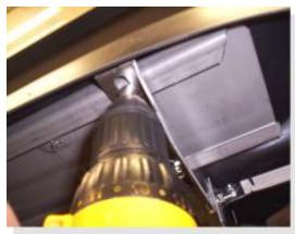
Position board where you want it, with the short step section towards the front. Install self tapping bolts through bracket into the shoulder of the steel channel on the bottom of the board. Level board and tighten any and all bolts. Repeat for other side.
