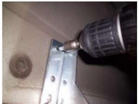
Attach 3124F to FL105 with two 5/16 nuts and bolts, snug but do not tighten yet. Attach brackets to vehicle by inserting the 5/16" bolt and nut through the pinch weld. Then install the self tapping bolts through the brackets into the body.
