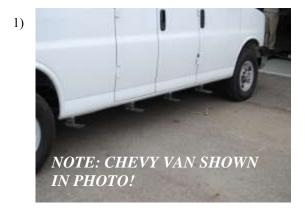
Measure from front wheel well back and make a mark at: 7",32",64",92" along the pinch weld. For 40" boards just use the 7", and 32" measurements.
