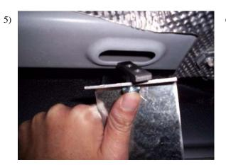
At the 37 3/4" mark on the pinch weld, look at the frame rail and you see a large oval factory slot, install bolt through slot on <u>FL 161 bracket</u>, attach re-enforcement nut to bolt and place in frame slot as shown above, make sure re-enforcement nut is straddled over slot and does not fall into slot of vehicle frame.
