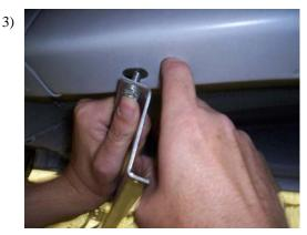
Thread 5/16" bolt through the rear slot of the <u>FL160 bracket</u> and into re-enforcement nut, as shown you will have to hold nut with finger to keep it from moving around on you.
