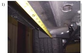
Measuring from the front wheel well, measure towards the rear of the vehicle. At locations 11 1/2", 37 3/4" and 66 1/4"" make a mark on the pinch weld, from there look at frame and you will find factory holes. These measurements are used for frame hole location only
