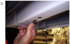
At the 11 1/2" mark (front), there are 2 factory holes on the frame rail. Slip the 2" x 1/2" reenforcement nut into the front slot.
