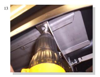
Once board is located left to right and is straight you are ready to attach board to brackets. This vehicle being so low to the ground ,you have to mark bracket slot locations rather than drill them on the vehicle. Fig.# 13 shows screws being run in with board on vehicle
