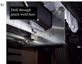
10 Straighten bracket as shown, snug bolt to frame. Drill through pinch weld and bolt bracket through the hole, again be sure not to drill hole to low. Tighten all bolts and nuts. IN405
