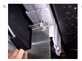
9) At the 66 1/4" look to the frame and you'll see a small slot to the front side of the leaf spring bracket. Put bolt through slot of bracket FL 162, then attach re-enforcement nut to bolt ( use tapped hole closest to end of nut on this Bracket to be able to install nut in hole as shown above.
