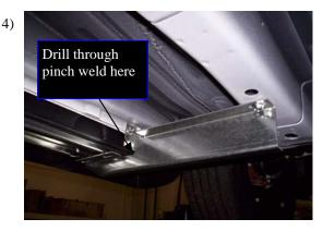
Straighten bracket, snug bolt to frame, and drill through where shown above. Be sure <u>not</u> to drill hole too low, as this will leave little or no steel on the pinch weld. Tighten both bolts as shown.
