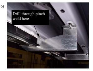
Straighten bracket as shown above, snug bolt to frame. Drill hole through pinch weld and bolt bracket to it. Be care full not to drill hole to low on pinch weld. Tighten bolts.
