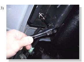
Remove the two forward bolts of the rear control arm holder. Do not discard, these will be used to attach rear bracket.
