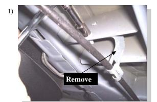
On the driver side at 25" (23" on passenger side) back from wheel well, remove factory bracket holding the emergency brake cable.
