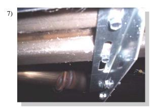
Place the board on the brackets. Using a small jack to hold the board, position it up against the vehicle to achieve the best fit. Slide the channel brackets up to the bottom of the board and attach with self drilling screws. Tighten the bolts holding the channels..
