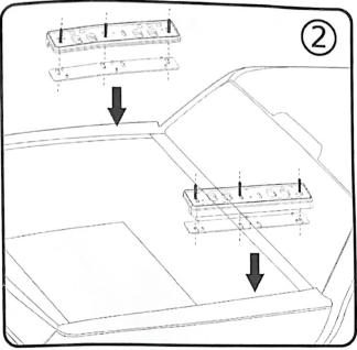
Slide the T-shaped screw into the groove, and then adjust the base to a suitable position on the car. The screw corresponds to the hole position, and then fixed and locked.
