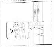
Loosen ①② screws properly, do not loosen all screws.
