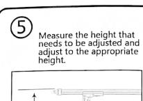
Loosen the screw on the post, adjust to the desired height, and observe the position of the scale value.
