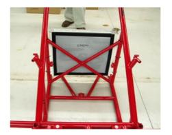
3.Once the Speed Screen is attached to the chassis, tighten down all Zip Ties drawing the Speed Screen nice and taut.
