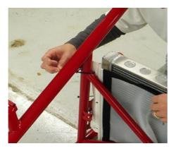
2. Using a Zip Tie through the holes in the rail strip, loosely attach to the chassis of the car. starting with the top above the cross member on both sides, and then the middle on both sides, and then the bottom on both sides.
