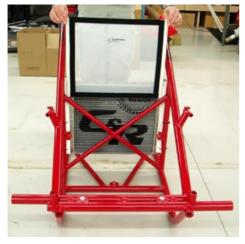
4. With the Speed Screen firmly attached to the chassis, the screen can now fully protect the radiator and be easily removed and re-installed for cleaning.
