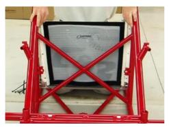
1. Starting with the Speed Screen and Rail together, place the <u>Speed Screen system</u> behind the air dam cross member.
