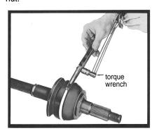
**STEP 3:** Place a wrench on the nut and draw the band up tight; then torque nut to 65 inch pounds as shown in photo above.
