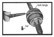
**STEP 5:** Back tool off just enough to permit tapping the band with a hammer until it lies flat across the top of the retainer, as shown in photo above. Tap the tabs of the retainer down until they fasten the strap securely, as shown in photo below.
