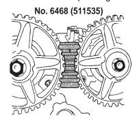
**3.** Follow vehicle service manual procedure to service timing belt as required. Remove tool when finished.
